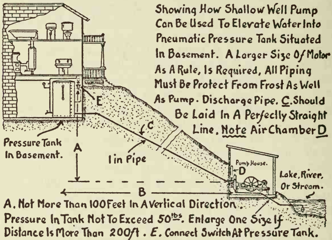
Fig. 2. Electric pumping of water to pressure tank.
